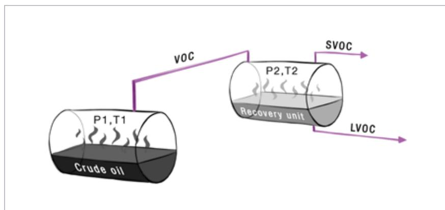
Fig. 1: Schematic showing VOC recovery
