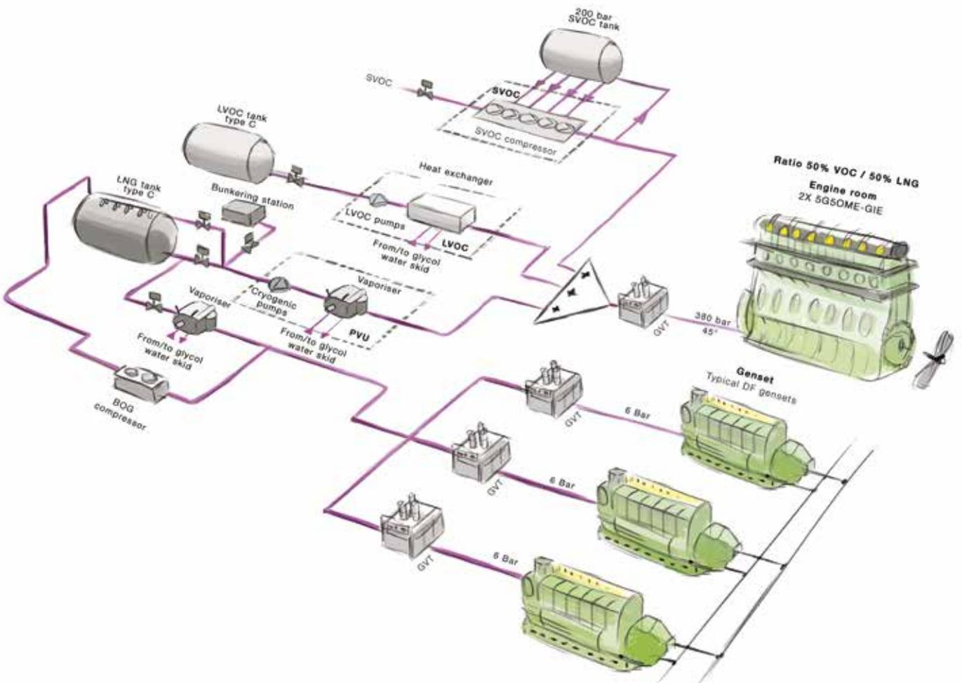
Fig. 3: FGSS where the recovery unit separates the VOC into LVOC and SVOC, which are mixed and burned in the ME-GIE in a predefined ratio
