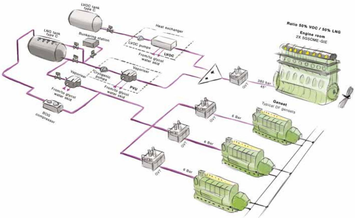
Fig. 2: FGSS for the LVOC burning ME-GIE two-stroke engine
